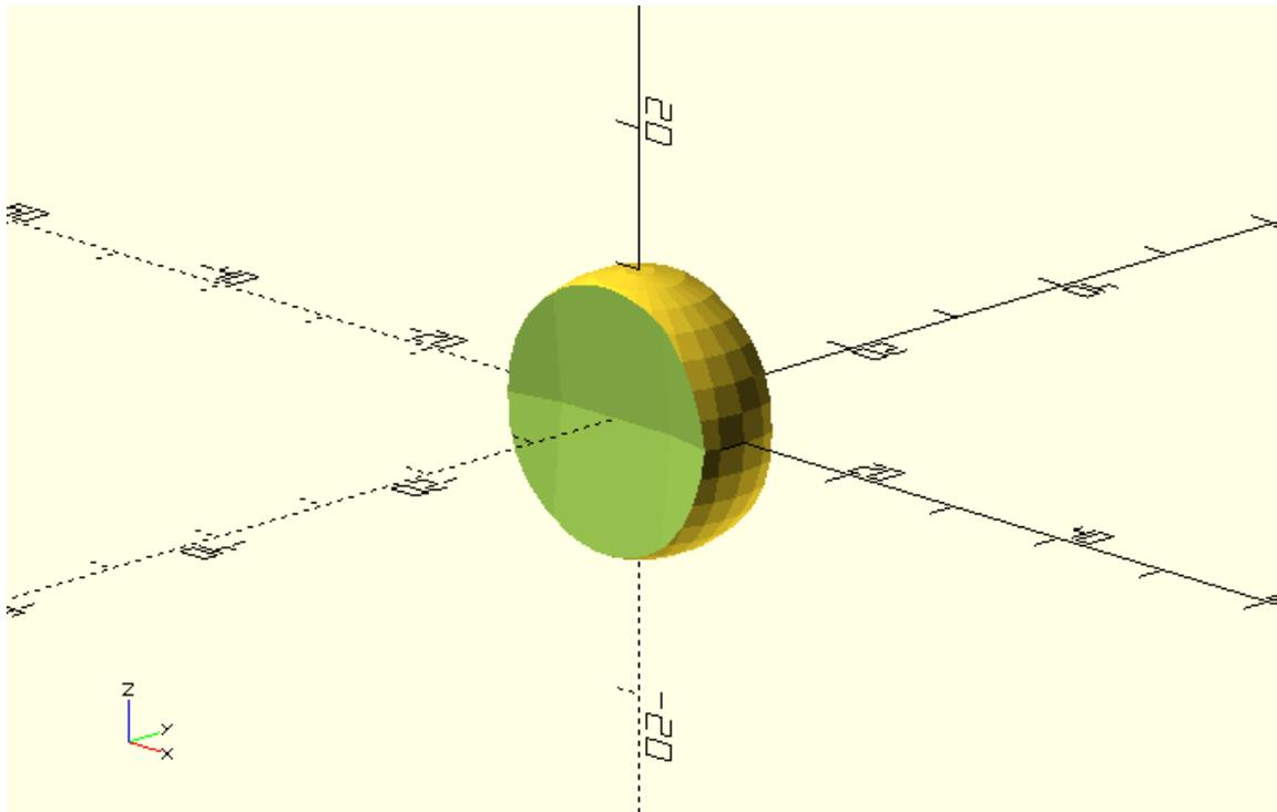
Try removing some material from the wheels by subtracting four cylinders that are perpendicular to the wheel. The cylinders should be placed at half the wheel radius and be equally spaced. Introduce a `cylinder_radius` and a `cylinder_height` variable. The value of `cylinder_height` should be appropriate so that the cylinders are always longer than the thickness of the material they are removed from.
