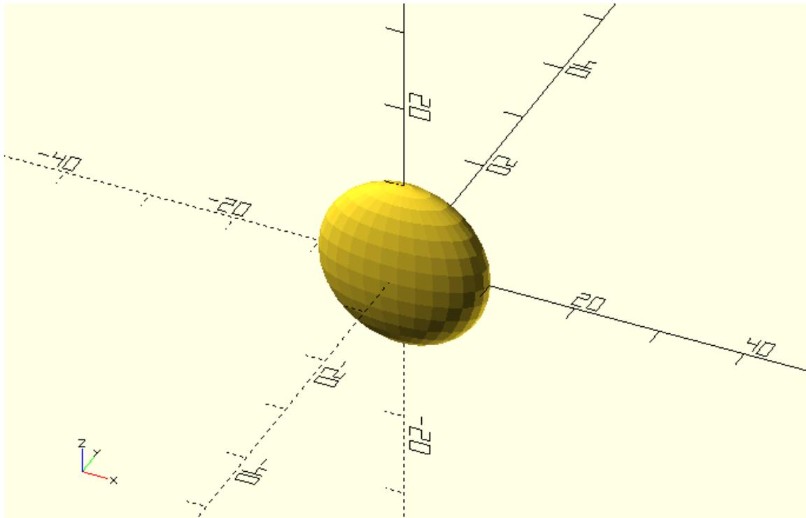
When you are scaling/resizing an object and you are concerned about its resulting dimensions it is more convenient to use the resize command. In contrast when you are concerned more about the ratio of the resulting dimensions compared to the starting dimensions it is more convenient to use the scale command.
