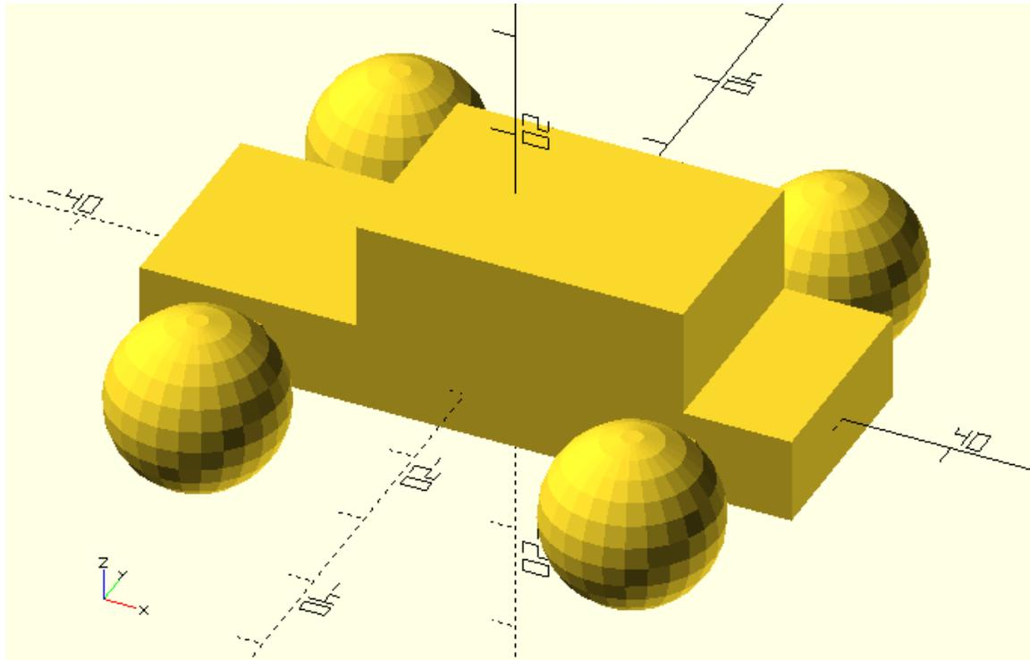
The idea to use a sphere to create the wheels was nice. You can now squish the spheres to give them a more wheel like shape. One way to do so is using the scale command.
