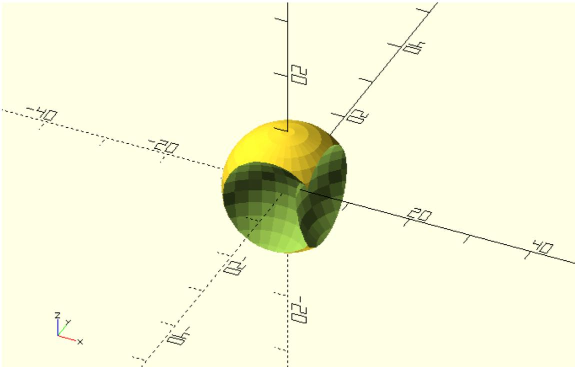
The third boolean operation is the intersection. The intersection operation keeps only the overlapping portion of all objects. The previous example results in the following model when the intersection operation is used.
