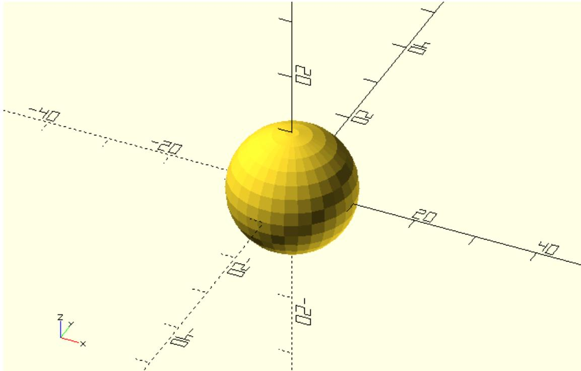
You should notice that the sphere is created centered on the origin. The input parameter `r` corresponds to the radius of the sphere.
