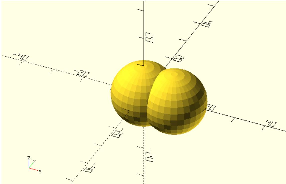
You should notice that the union command doesn't have any input parameters. This is true for all boolean operations. The union is applied to all objects inside the curly brackets. You should also notice that the statements inside the curly brackets have a semicolon at the end. In contrast there is no semicolon after the closing curly bracket. This syntax is similar to the use of transformations when applied to multiple objects.
