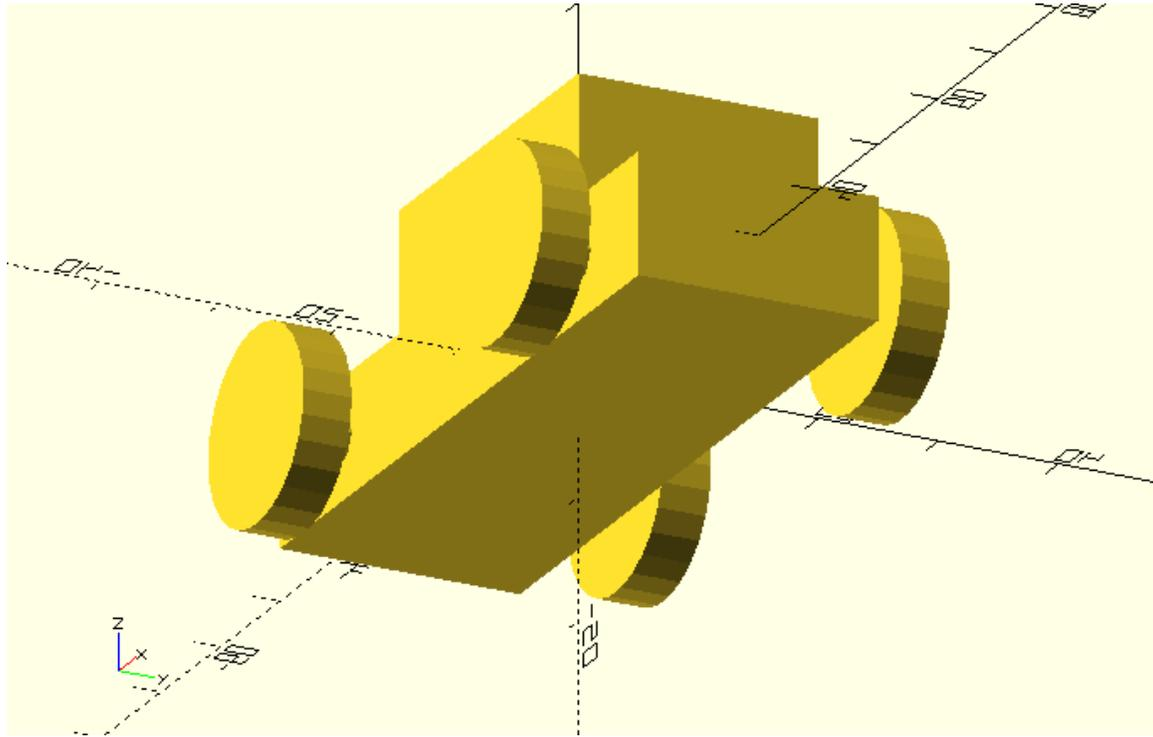
You should notice that a wheel is no longer created at the origin. You should keep in mind that the use command works like the include command with the only difference being that the use command doesn't create any objects, but rather just makes the modules of the external script available in the current script.
