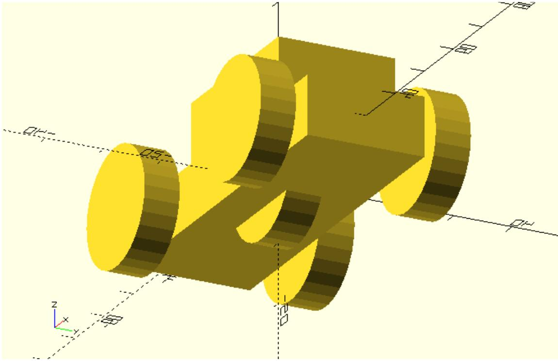
Define the `wheel_radius` and `wheel_width` parameters in the calls to the `simple_wheel` module. To do so use the existing `wheel_radius` variable as well as a `wheel_width` variable that you are going to define. Set the variables equal to values that you like.
