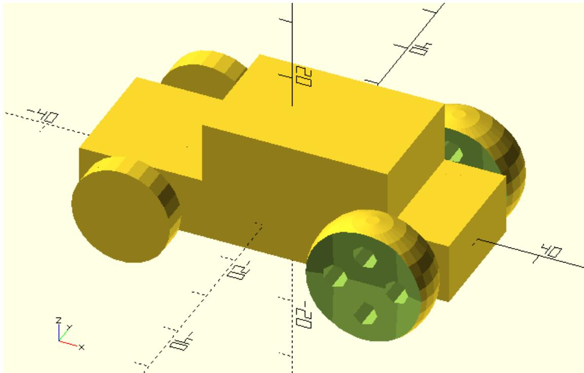
With this example it should be clear that the name of the script doesn't have to be the same as the name of the module as well as that a script can contain multiple modules. There is no right or wrong way on how you should go about organizing your library of modules. In the last example a wheel.scad script which defines the different wheel modules was used. Alternatively you could have saved each module as a separate \*.scad script.
