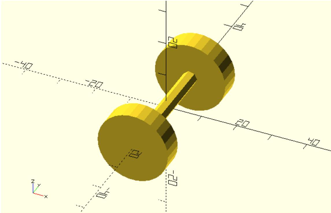
If you simply wanted to only use the above set of simple\_wheels, that approach would be just fine. The problem though is that this axle\_wheelset module is not really flexible and parameterizable to the desired degree. On one hand you can customize all input parameters, but on the other hand, could you swap the simple\_wheel design with the complex one? The fact is that with the above approach in order to do so you would have to define a completely new module.
