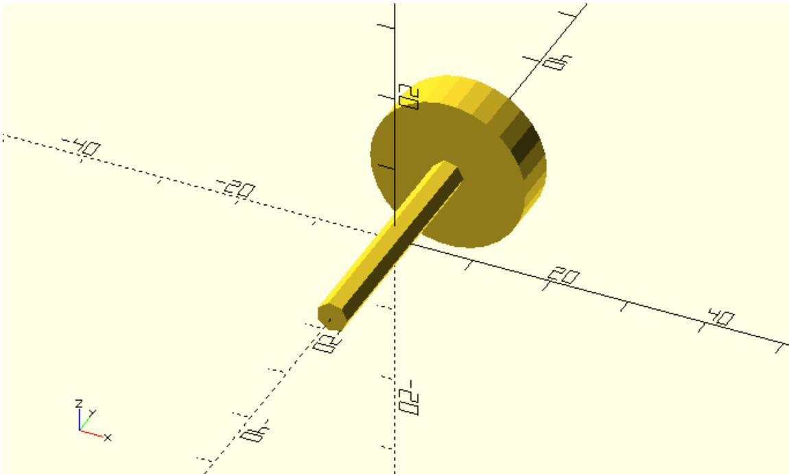
Add an `axle_wheel` module on the `vehicle_parts.scad` script. Make use of the `children` command to parameterize the specific choice of wheel design. Use the `vehicle_parts.scad` script on another script to create any vehicle design that you like.
